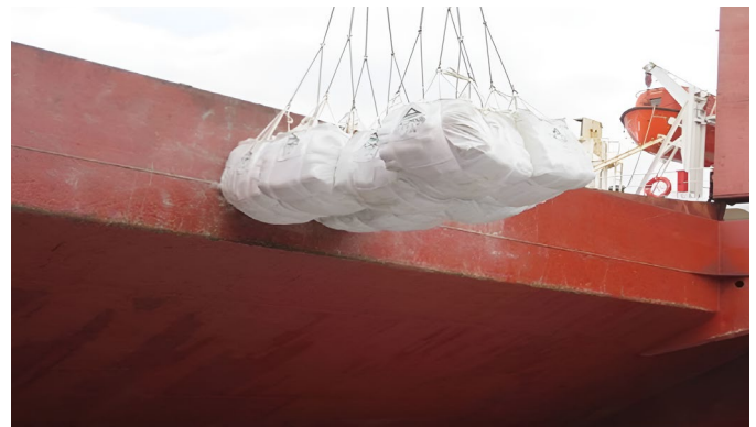
FIGURE 6 Banging of the bag on the hatch coaming during discharging
