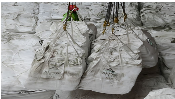
FIGURE 8 Incorrect hooking FIBC bags
