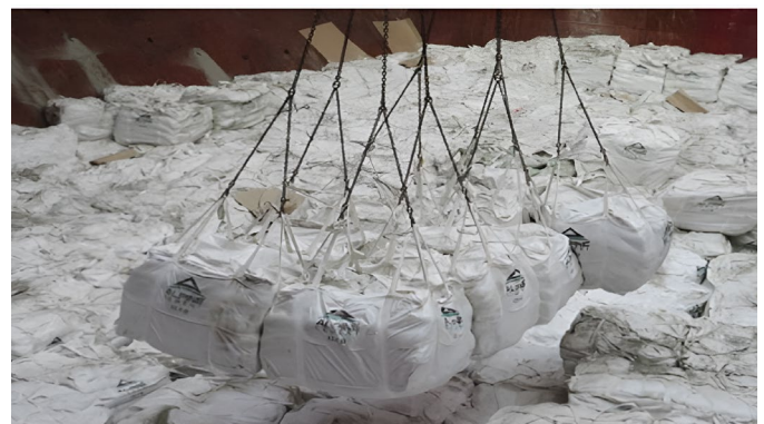
FIGURE 9 Correct way of hooking FIBC bags
