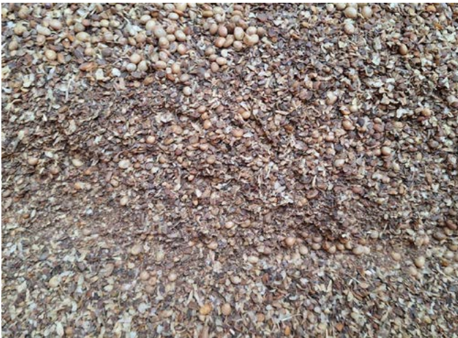
FIGURE 3 Localised foreign matter and dust often leads to development of hotspots. Above shows a caked area hotspot with high foreign matter content and darker discolouration.
