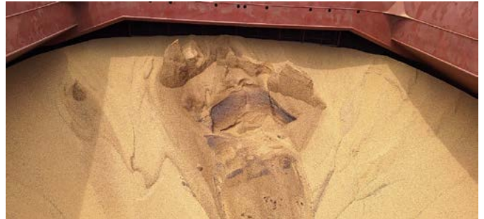
FIGURE 5 Heat-damaged layer present in a cargo of soya beans. The dark central layer contained high concentration of other mixed types of grains and foreign matter indicating the loading of a contaminated parcel.
