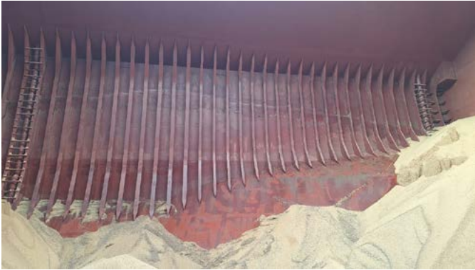
FIGURE 7 Mouldy cargo residue left on side steelwork related to a surface mould crust
