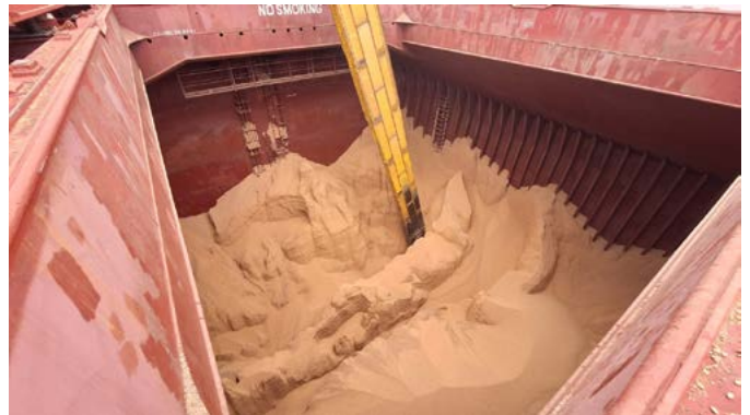
FIGURE 6 Deep seated caking present in soya bean cargo discharged by unloader
