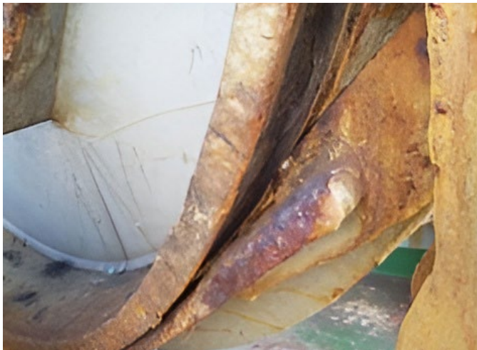
FIGURE 12 Worn brake lining
