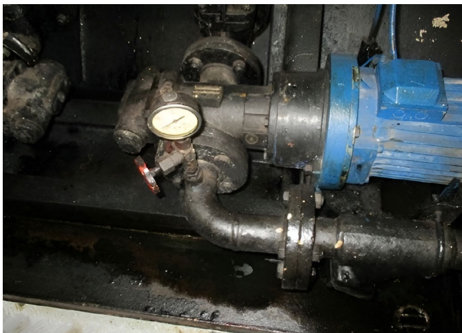
FIGURE 16.2 Oil leaks in engine room
