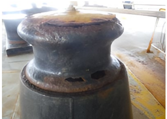
FIGURE 14 Fairlead in poor condition
