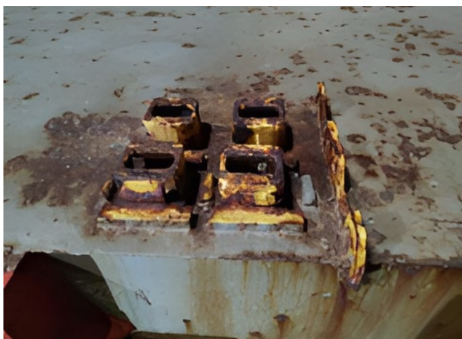
FIGURE 1 Corroded container securing points
