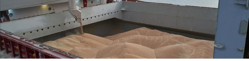
To address this, the new amendment recognises this specific loading condition and requires the Grain Loading manual to include the corresponding heeling moment values for such scenarios. This will allow an exemption from trimming the ends.
