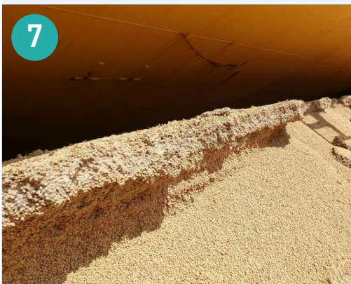
Figure 7: A close up of surface mould crust associated with self-heating within the stow of soya beans. Moisture condenses in the relatively cooler upper layer of cargo leading to mould growth which often forms a white layer of mould.
