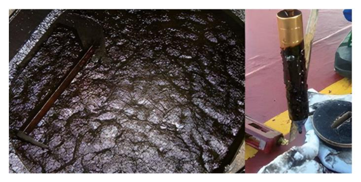
Remaining vigilant is key to identifying and mitigating the risks associated with the Cappuccino Effect. The following signs may help in recognising such instances during bunkering operations:
