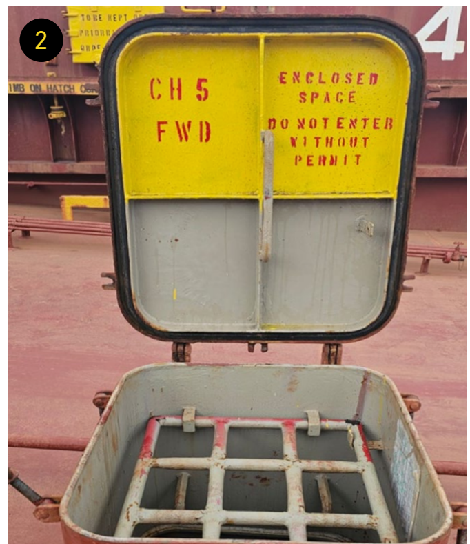
FIGURE 2 EXAMPLE OF WARNINGS ON BOOBY HATCHES
