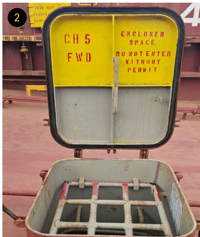
FIGURE 2 EXAMPLE OF WARNINGS ON BOOBY HATCHES
