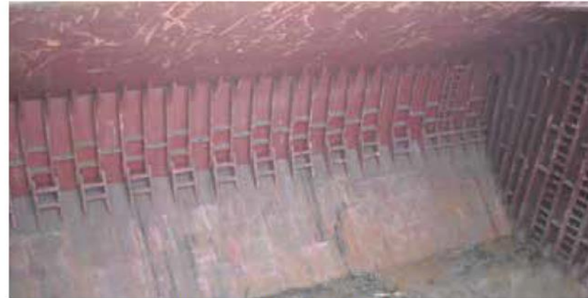
✗ Unprepared cargo hold on a bulk carrier. Residue from some cargoes can react with, and damage, steel cargo and should be cleaned in line with the applicable MSDS requirements
