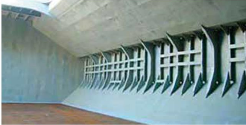
✓ A bulk carrier cargo hold in a clean condition ready for loading. Dryness of the cargo hold is an important factor in prevention of corrosion/rusting
