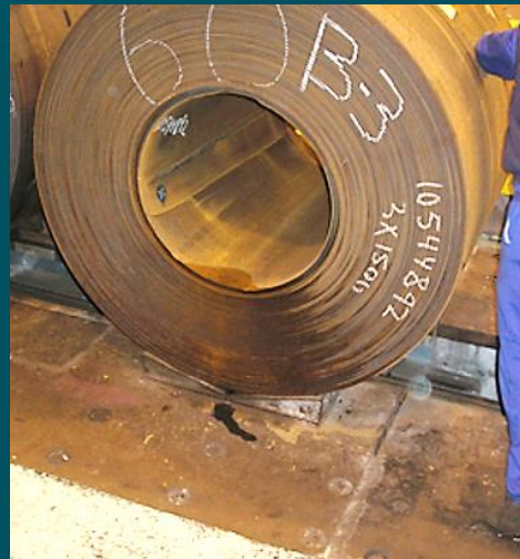
Water along coil layers draining to and out of the bottom of the coil. Dark patch on concrete is a silver nitrate test
