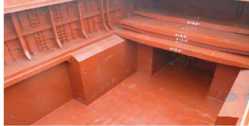
✓ A cargo ship with box-shaped cargo holds and pontoon 'tween deck ready for loading
