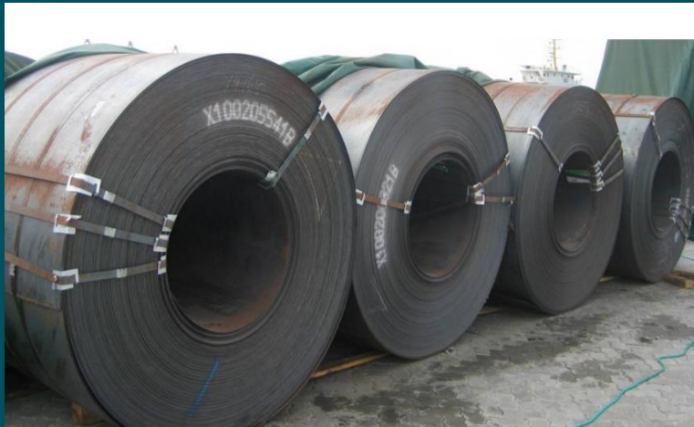
Bands were too slack & moved
