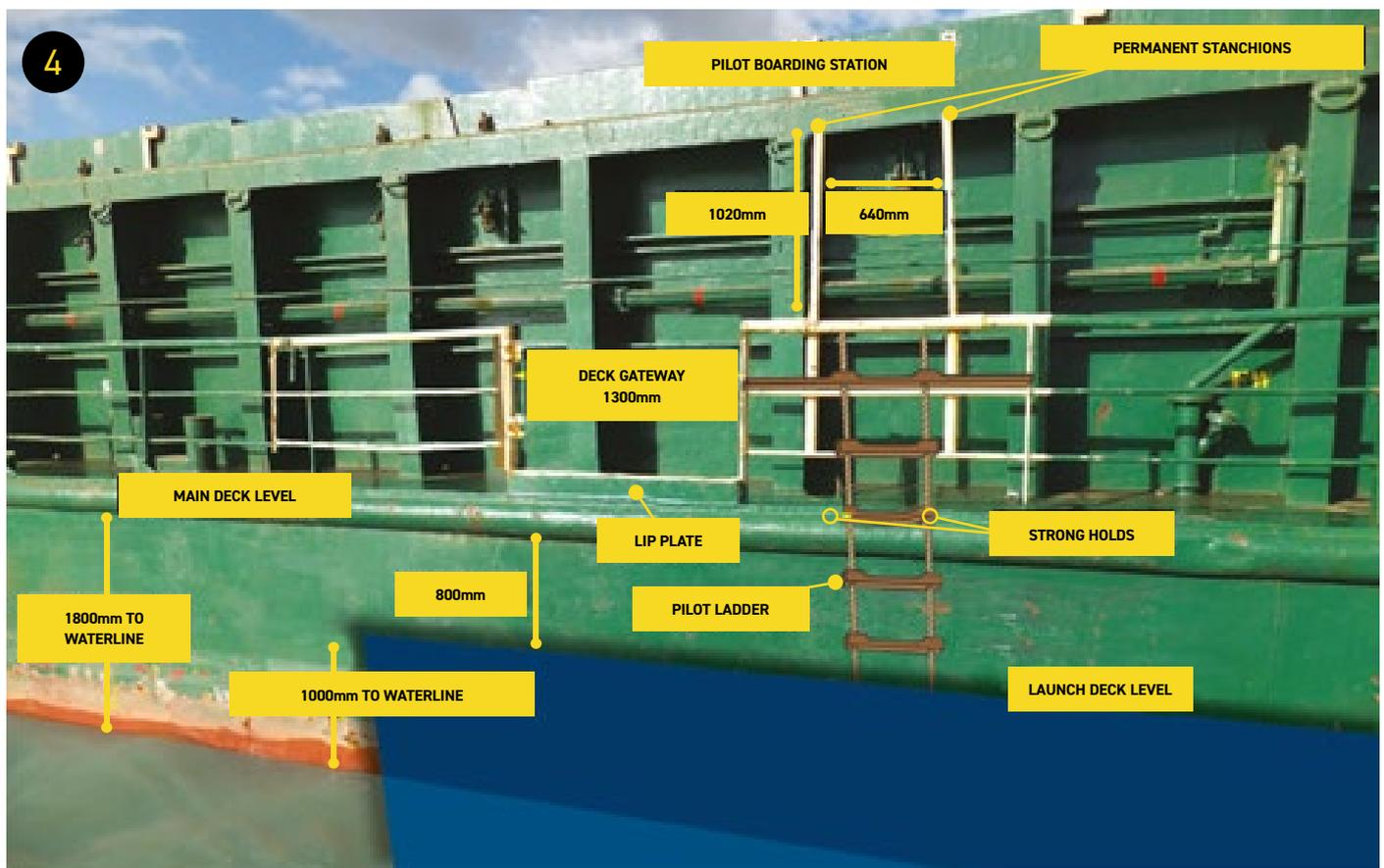
**FIGURE 4** REPRODUCED IMAGE OF CARGO VESSEL'S DECK GATE AND PILOT BOARDING ARRANGEMENTS
