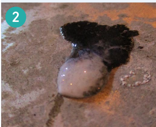
Figure 2: When in contact with chlorides, silver nitrate solution changes from a clear solution to being milky.
