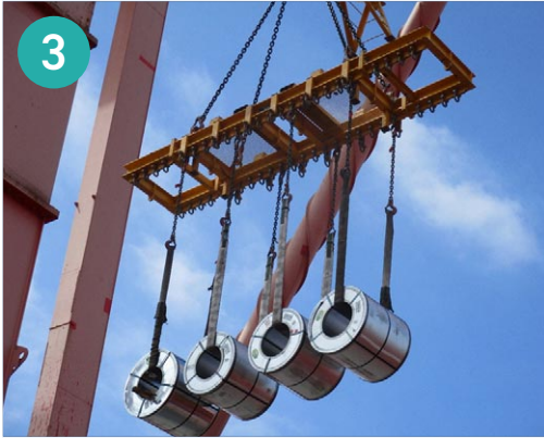
Figure 3: Multiple CRCs being lifted by webbing slings.
