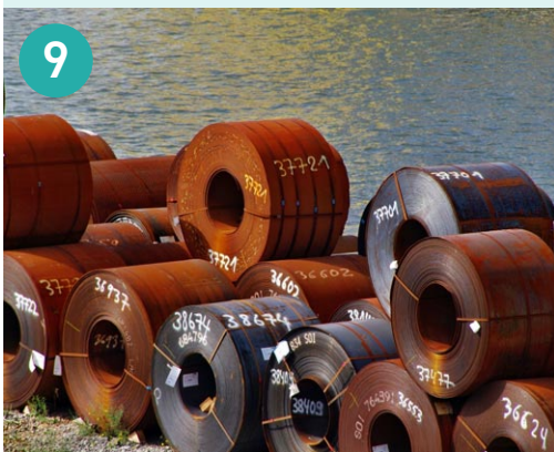
Figure 9: Hot Rolled Coils (HRC) are uncovered, and as they are often stowed outside briefly, light rusting is not unusual. Heavy rusting as seen on most of these coils is not acceptable.
