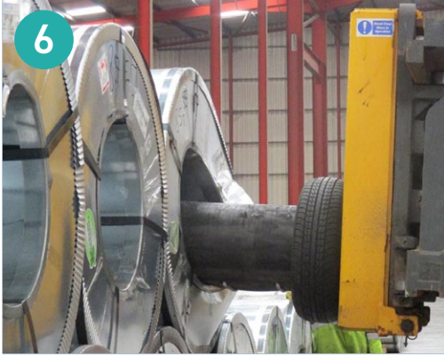
Figure 6: Handling damage caused ashore should be carefully recorded, noting whether the steel product is damaged, or just the covering where fitted.
