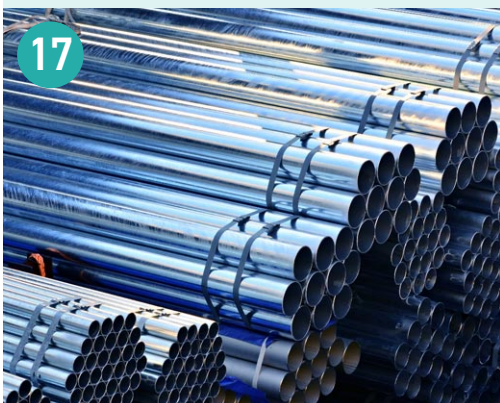
Figure 17: Pipes are usually bundled, with the ends in particular being susceptible to damage.
