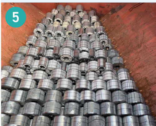
Figure 5: Stowage and securing in end cargo holds can be more challenging due to their shape.
