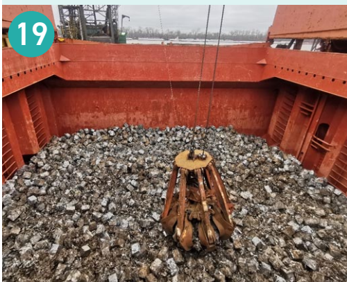
Figure 19: Ensure scrap presented for loading is as permitted by the charterparty, because there are many different specifications.
