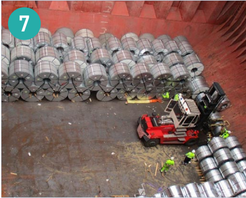
Figure 7: Discharge of CRC. Note the dunnaging under the coils and the lashing of the coils into a tight homogenous stow using steel banding.
