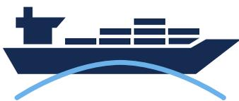
Vessel rolls to one side whilst on the wave crest, stability decreases and large roll motions are experienced.
