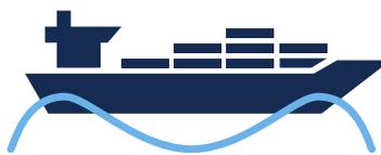
As Vessel uprights on the trough of the wave, stability increases leading to a strong push, worsened by a high GM / stiff vessel.
