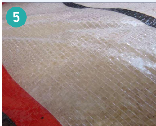
Figure 5: Condensation on interior of bag following exposure to direct sunlight during discharge.
