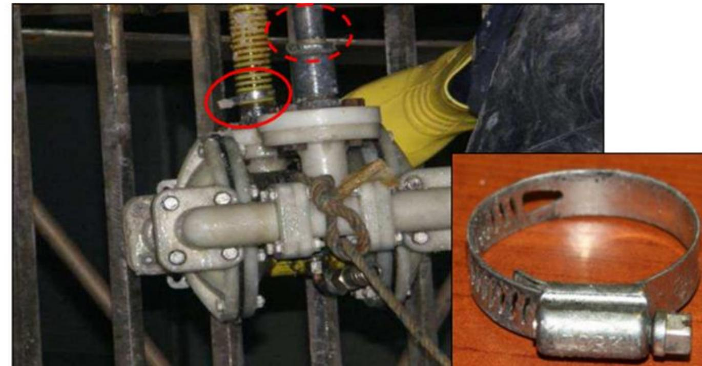
Remaining hose clamp on the suction line and a sample clamp.
