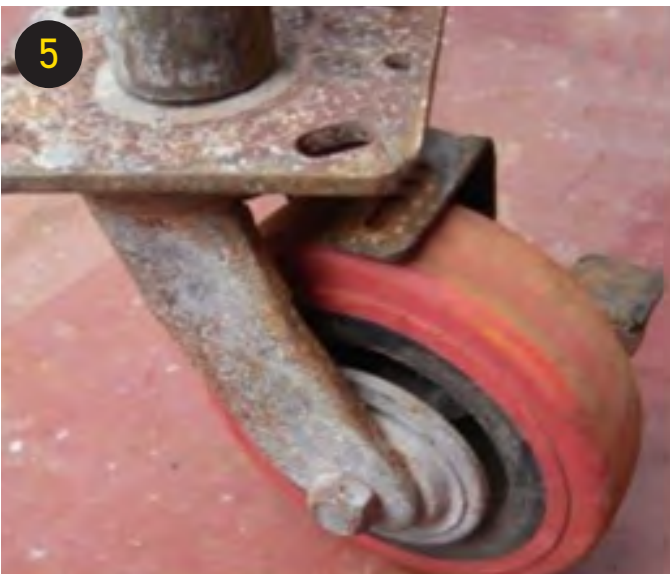
FIGURE 5 INOPERATIVE SCAFFOLDING SWIVEL WHEEL BRAKES ON THREE OF THE FOUR WHEELS. SOURCE: AUSTRALIAN TRANSPORT SAFETY BUREAU (ATSB)
