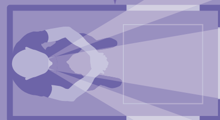
Plan view of watch room showing deckhand's limited visibility when sitting with his back against the wall
