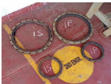
Damaged 'O' rings due to corrosive nature of the cargo.
