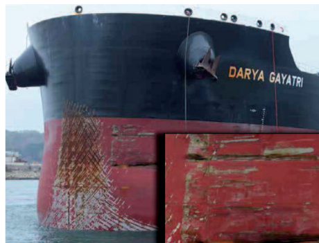
Damage to DARYA GAYATRI and PAULA C
