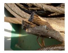
A general cargo ship was fitted with twin cranes between nos. 1 and 2 cargo holds. During the discharge of an item of project cargo weighing 27mt, which was within the safe working load of the crane and the wire, the steel hoisting wire failed. The project cargo fell down into the hold and damaged other items of cargo as well as causing damage to the ship's tween deck.
