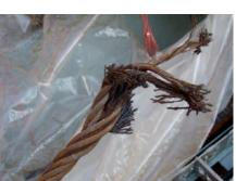
Classification society surveyors can only spend a limited time on board looking at the whole ship and crew and shore staff must be aware that inspection of the crane wires may be visual only and will not usually involve a close examination of the core of the wire. Therefore, they should make their own, systematic, assessment of the condition of ship's crane or derrick wires at regular intervals.
