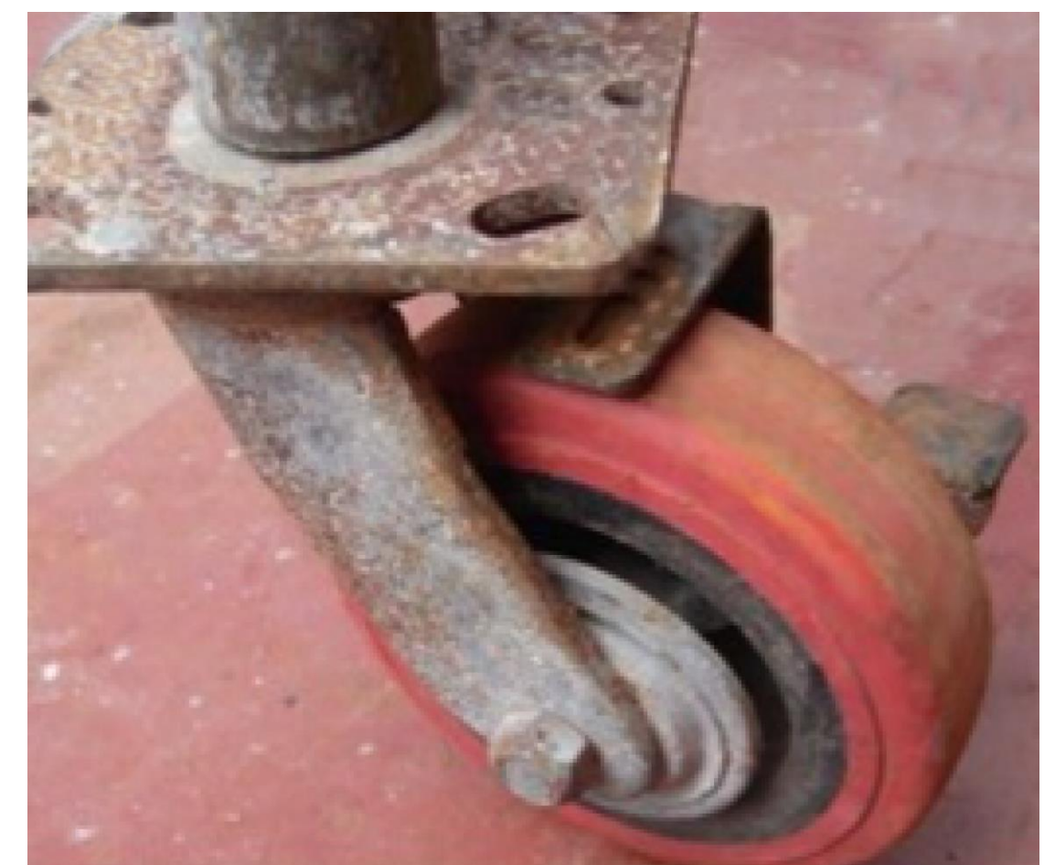
Inoperative scaffolding swivel wheel brake
