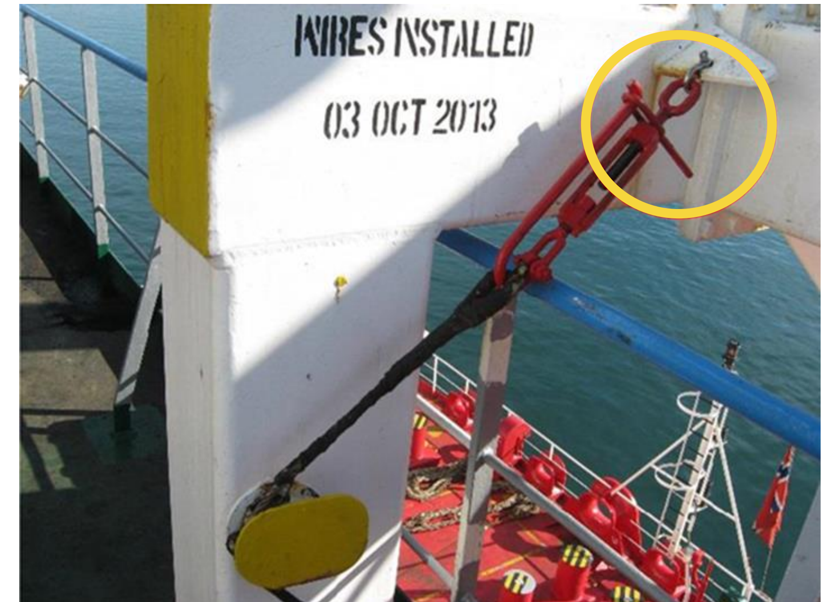
Turnbuckle and the pin (marked with yellow circle) after the maintenance job completed.
