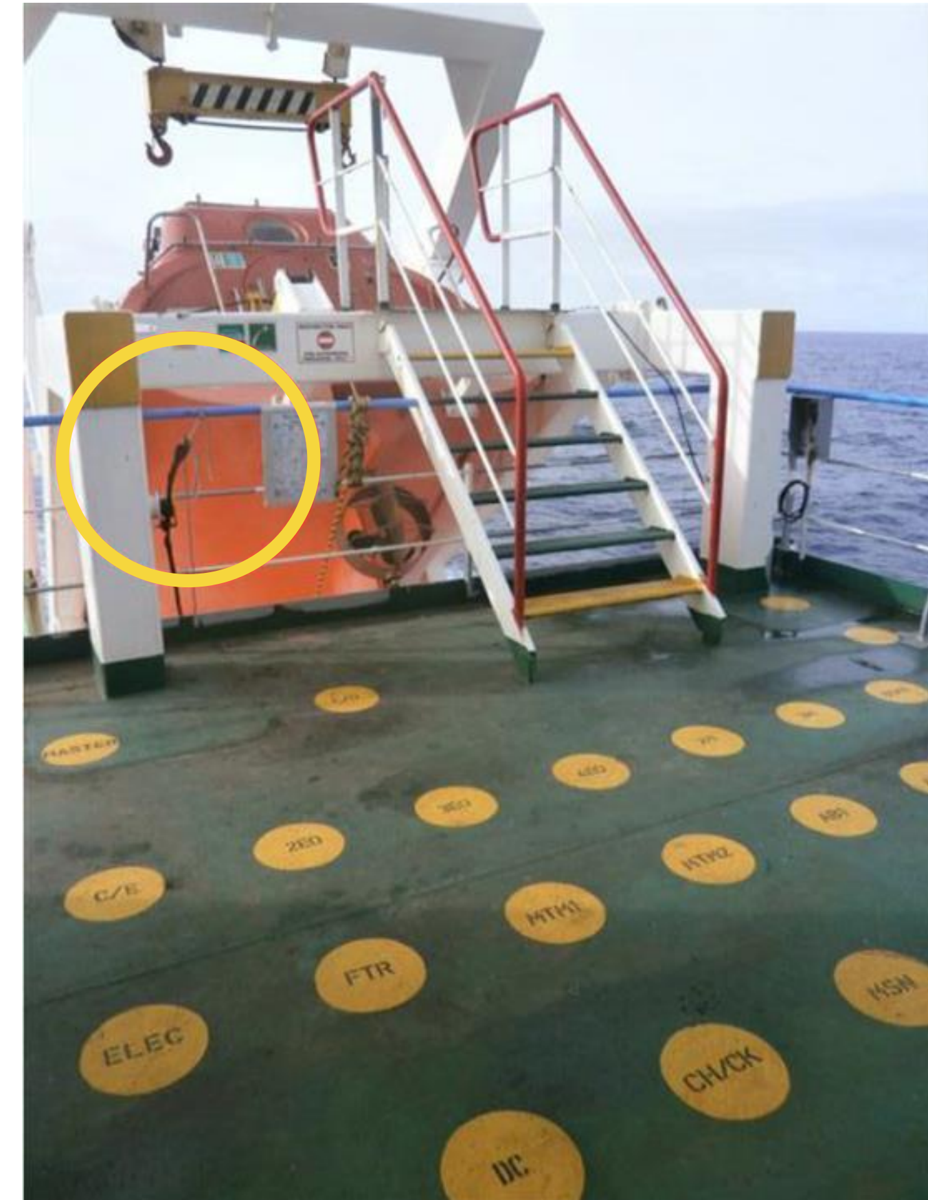
Working area for the original maintenance task (turnbuckle marked with a yellow circle).
