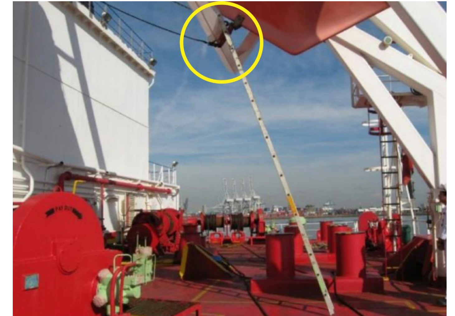
Free-fall lifeboat and forward hook (marked with a yellow circle) with ladder as positioned by the AB
